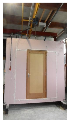
Door assembly incorporating R w EX™ sealing systems undergoing independent smoke performance testing
