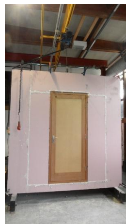
Door assembly incorporating R w EX™ sealing systems undergoing independent smoke performance testing
